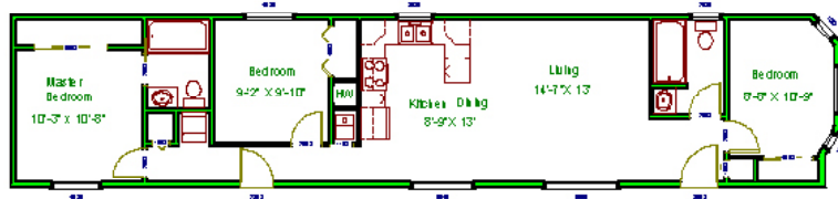
14'x66' Single Wide Floor Plan - Savannah Series Model 301, 924 sq ft
